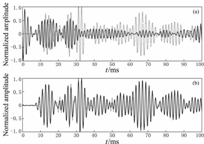
**Figure 5** (a) True Green's function (dotted line) and the Green's function estimated from the cross correlation of waves excited by a single source (solid line); (b) True Green's function (dotted line) and the Green's function estimated from the cross correlation of waves excited by 300 sources placed uniformly on a circle (solid line).
