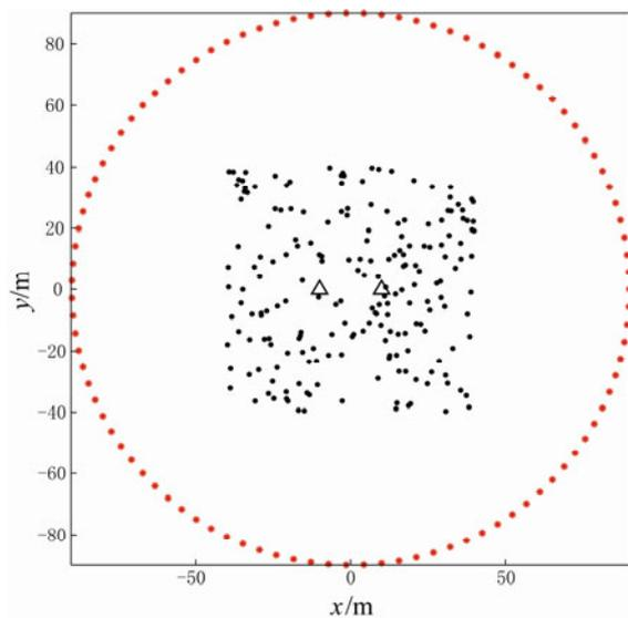
**Figure 4** Geometry for the numerical example of 2D scattering by 200 scatterers (dots) of waves excited by sources on a circle. Receivers are indicated by triangles. The scattering cross section of each scatterer, which is a length in two dimensions, is much larger than the radius of each dot.
