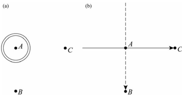
**Figure 1** (a) A point source in a homogeneous acoustic medium at point  $A$  that emits equal amounts of energy toward points  $B$  and  $C$ ; (b) Equal energy transport along the dashed and solid arrows is needed to retrieve the Green's function for the propagation from the source point  $A$  to the points  $B$  and  $C$ .
