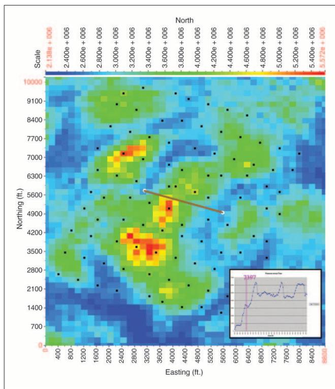
**Figure 8.** Depth slice at the reservoir level through an emission energy cube derived from one minute of observation time during a hydraulic fracture stimulation of a horizontal well. The hotter colors represent areas of higher energy acoustic emission. The energy distribution is consistent with fractures being set up in two directions (Figure 1 from “Reservoir characterization using surface microseismic monitoring” by Duncan and Eisner.)
