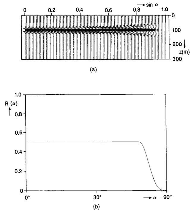
FIG. 5. Prestack migration with the correct source representation (Figure 2a). (a) Angle-dependent reflectivity image. (b) Angle-dependent reflectivity at  $z = 100$  m. Note that  $R(\alpha) = 0.5$  up to high incidence angles.
