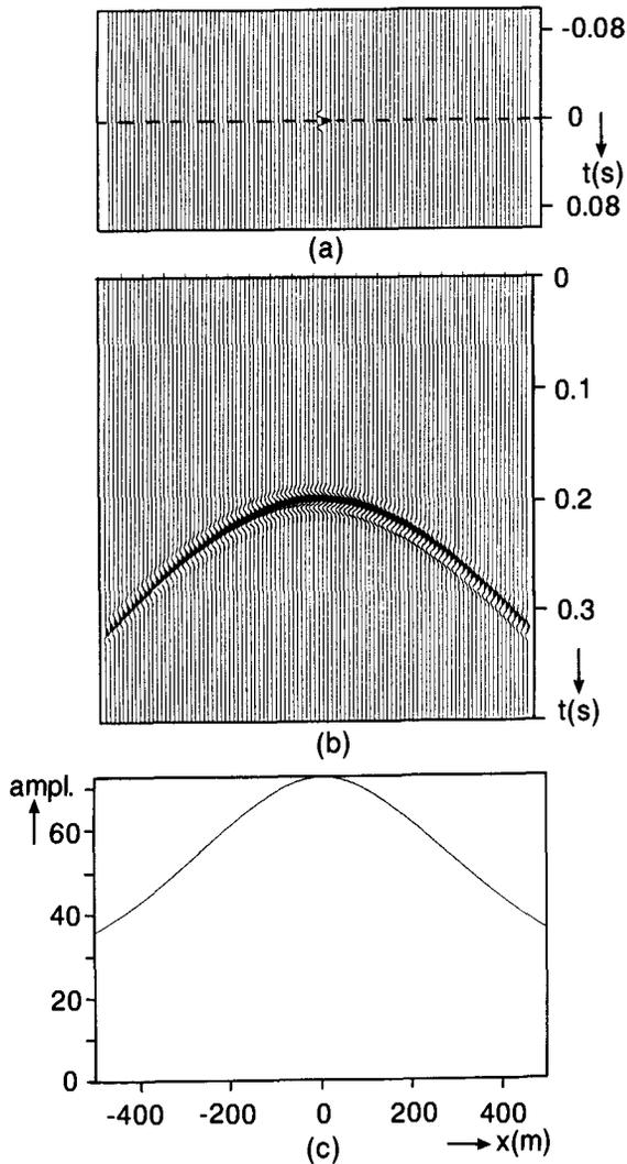
FIG. 1. Dipole source wave-field extrapolation. (a) One-way representation of a band-limited source of vertical force at  $\mathbf{r} = \mathbf{0}$ . (b) Downgoing wave field at  $z = 400$  m obtained by applying one-way wave-field extrapolation to the data in (a). (c) Amplitude cross-section of (b).
