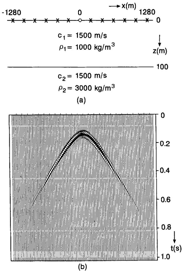
FIG. 3. Model for evaluating angle-dependent reflectivity imaging. (a) Subsurface configuration with a density contrast at  $z = 100$  m,  $R(\alpha) = 0.5$ . (b) One-shot record for a monopole source at  $(x = 0, z = 0)$ .
