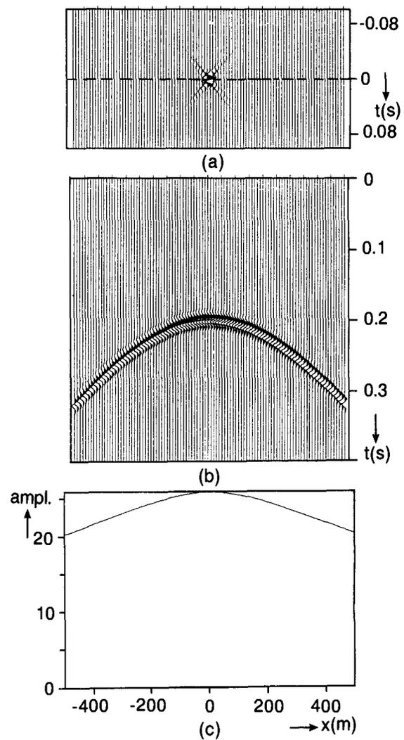
FIG. 2. Monopole source wave-field extrapolation. (a) One-way representation of a band-limited source of volume injection at  $\mathbf{r} = \mathbf{0}$ . (b) Downgoing wave field at  $z = 400$  m obtained by applying one-way wave-field extrapolation to the data in (a). (c) Amplitude cross-section of (b).
