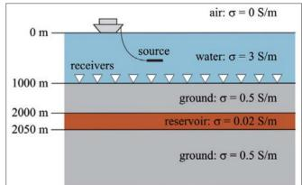
**Figure 2.** The modeling setup (not to scale). The source (black horizontal bar) is 25 m above the receivers (white triangles). The electric conductivity  $\sigma$  is given in every layer.
