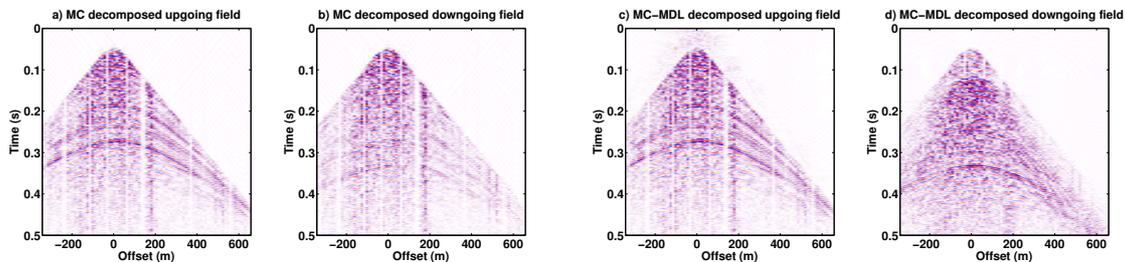
**Figure 2** (a) Upgoing, MC decomposed fields. (b) Downgoing, MC decomposed fields. (c) Upgoing, MC-MDL decomposed fields. (d) Downgoing, MC-MDL decomposed fields.
