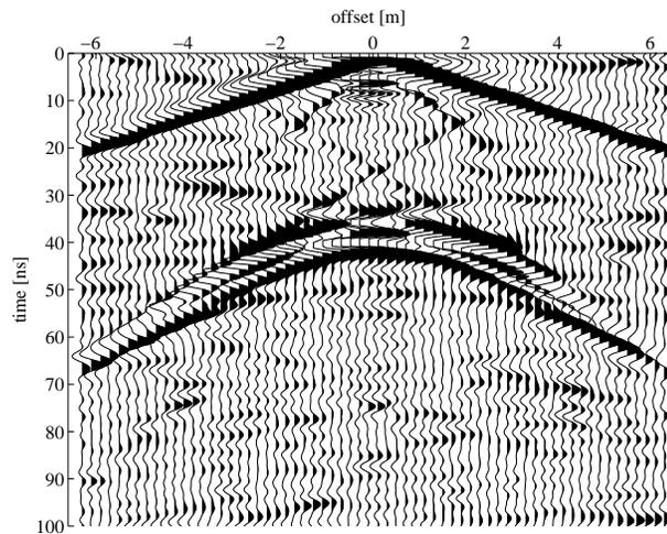
Fig. 4. A two-sided CMP constructed using only noise sources in the upper half space with the midpoint directly over the syncline, with 20 cm stepsize.
