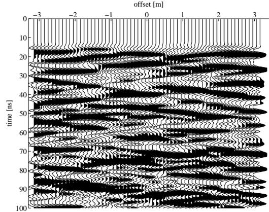
Fig. 2. The first 100 ns of a noise recording from sources in the upper half space only, with 10 cm distance between the recorders. A two-sided CMP, with  $x = 0$  as midpoint, can be constructed by autocorrelating the midpoint trace and subsequent crosscorrelating a recording at negative distance with one at the same positive distance.
