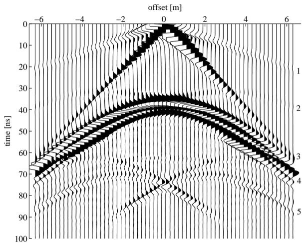
Fig. 3. A two-sided CMP directly modeled with the midpoint directly over the syncline, with 20 cm stepsize.
