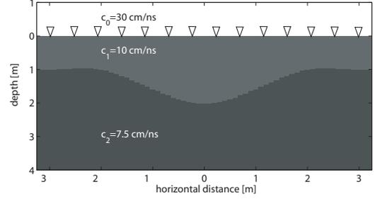
Fig. 1. The model used for the example with noise sources. It has a syncline in the first layer.
