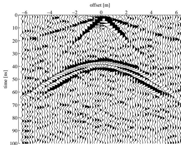
Fig. 5. A two-sided CMP constructed using noise sources in the upper and lower half spaces with the midpoint directly over the syncline, with 20 cm stepsize.
