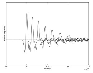
Fig. 3: Transmission responses (convolved with Ricker wavelet) for varying impedance contrast.
