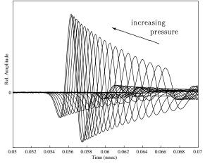
Fig. 1: Transmission responses of Rotliegend reservoir sandstone for varying ambient pressure.
