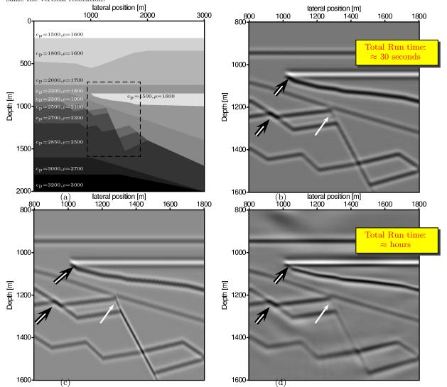
Fig. 7: (a) Graben model. Velocities in m/s and density in  $kg/m^3$ . The following zoomed in sections: (b) Simulated migrated section using resolution function at 1200m from velocity trace at 1200m. (c) 1D method. (d) Finite difference modeled and migrated section using the true velocity model. See text for more details.
