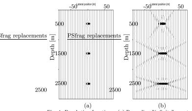
Fig. 4: Resolution functions. (a) Recording "infinite" aperture and all propagation angles. Note that almost the same result would be obtained with the 1D convolution model. (b)  $\alpha_{max} = 60^o$  and an aperture width of 3000 meters. The 2D resolution function is "smeared" out and varies in depth.
