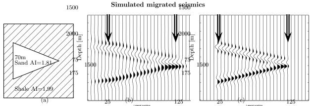
Fig. 6: (a) Sand wedge model. (b) Simulated migrated image of sand wedge placed at 1500 meters depth. (c) For comparison the 1D convolved sand wedge. The simulated migrated image shows a decrease in horizontal resolution (arrows) and approximately same the vertical resolution.
