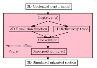
Fig. 2: Framework to obtain a simulated migrated seismic section. Summarized by convolving the resolution function with a reflectivity trace, followed by superposition of all convolution products for all reflectivity traces.
