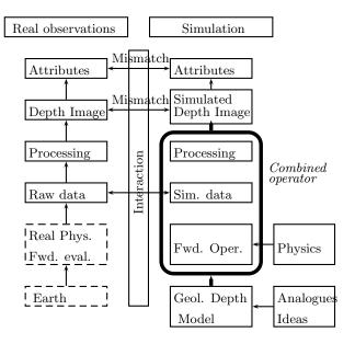
Fig. 1: "Simulation in a complete sense", modified after Petersen (1992). The combined operator, thick box, fits in this framework by acting as a direct transfer function from the Geological Depth Model to a simulated migrated Depth Image.
