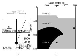
Fig. 3: (a) Acquisition setup with a limited aperture and selection of the maximum angle of propagation  $(\alpha_{max})$ . (b) Simple salt model, the asterisks denote the positions of obtained resolution functions.
