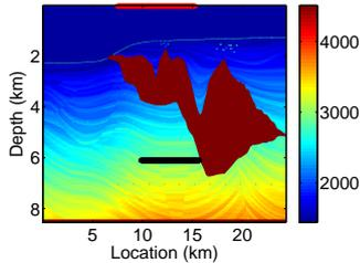
Figure 1: The Sigsbee model with an array of 128 sources at the surface in red and an array of 128 receivers in a horizontal well in black.
