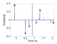
Figure 2: Image showing the result of step 1. The windowing function  $\Theta$  is indicated by the black vertical line. Left of the window: the upgoing focusing function. Right of the window: the upgoing Green's function.
