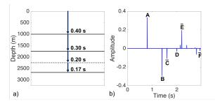
Figure 1: (a) Image of the layered 1D model with 3 interfaces. (b) Reflection response recorded at the surface.
