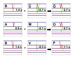
Figure 9: Illustrations of the events in the upgoing focusing function and Green's function after step 3. Events  $\overline{O}$  and P are found in the second term, while event O is a contribution of the third term.
