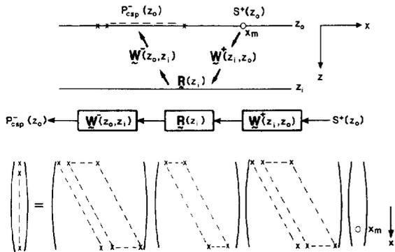
FIG. 3. Basic model for the seismic response from depth level  $z_j$ .
