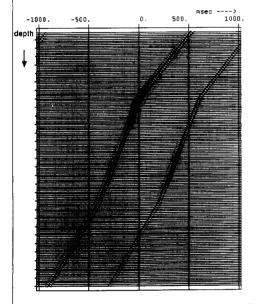
Fig. 2a. Multi-fold zero-offset panel for depth points situated on a vertical line. Using correct velocity for first layer yields focus at zero time and at reflector depth (400 m). Incorrect velocity in second layer results in focus off the zero time axis and not at reflector depth.
