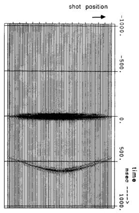
Fig. 3. Common-depth-point gather of a depth point at 400  $\,\mathrm{m}.$
