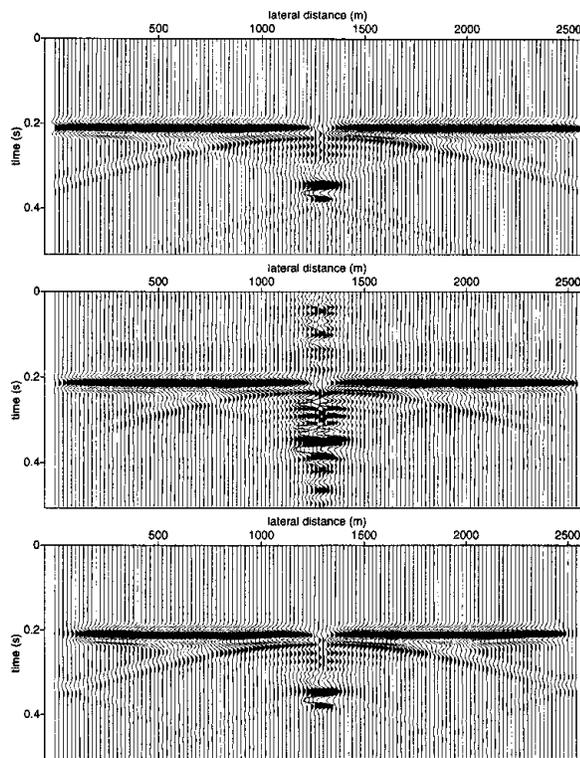
Figure 5: Results of 1000m extrapolation: finite difference (top), standard method (middle) and modal decomposition (bottom).
