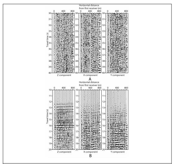
**Figure 1. (A)** Ten seconds of seismic background noise as recorded by the vertical (Z), the horizontal in-line (X) and the horizontal cross-line (Y) components of the geophones. **(B)** Another ten seconds of seismic background noise.
