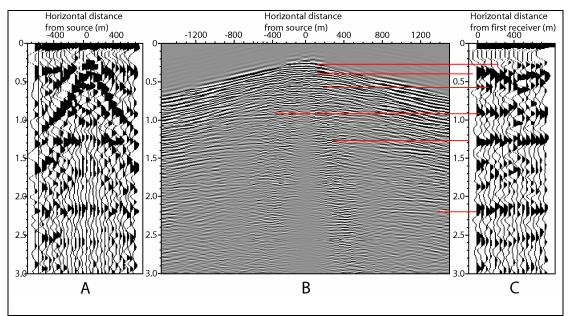
Figure 2. (A) Common-offset stack panel obtained from the common-source gathers retrieved from the passive data. (B) Common-offset stack panel after surface wave elimination in the active survey. (C) Line-source response obtained by summing the common-source panels retrieved from the passive data (brute stack).
