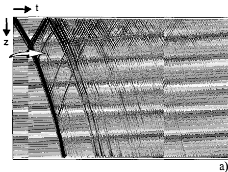
Figure 3.32 a) Finite difference modeling of the vertical zero-offset VSP ( v_z ) with the source at 1050m, b) acoustic layer parameters of the subsurface model.
