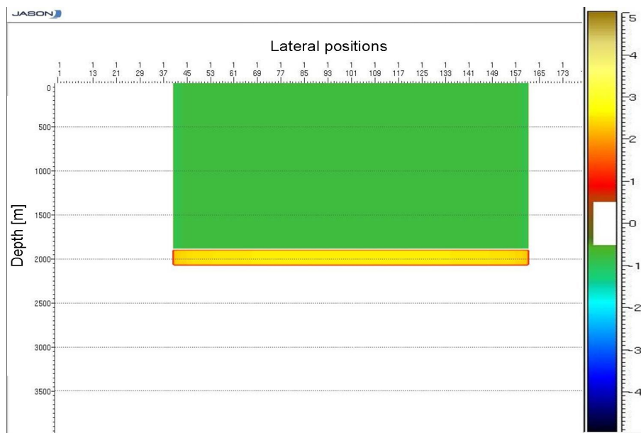
Figure 5.12: Relative changes in the P-Velocity (Model 1 - Table 5.1) in %, in the overburden and at the reservoir level, after pressure depletion of 15 MPa. Note that the colors represents the changes in the acoustic velocity in %.
