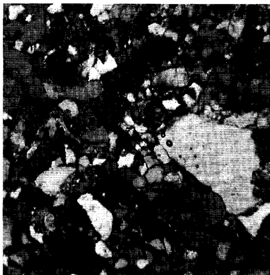
Figure 4.11: Thin section of the Niederhausen Rotliegend sandstone using polarized light. Orientation of the section is parallel to the layering.
