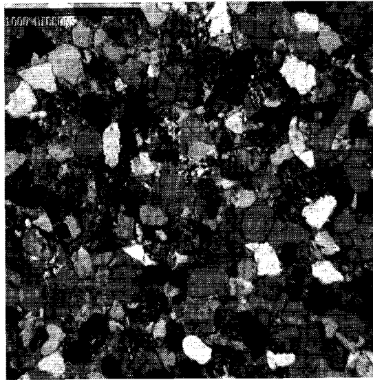
Figure 4.8: Thin section of the Flechtinger Rotliegend sandstone using polarized light, showing subrounded grains.
