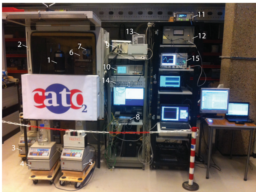
Figure 2.3: Experimental setup. 1 – sample in the pressure vessel, 2 – oven, 3, 4, 5 – ISCO pumps, 6 – density meter, 7 – pressure difference gauge, 8 – strip chart recorder, 9 – Agilent multiplexer switch, 10 – Wayne Kerr Precision Component Analyser 6640A, 11 – Agilent 33210A function generator, 12 – ENI 2100L RF amplifier, 13 – NI PXIe-1082 chassis with NI PXIe-7962R FlexRIO FPGA and NI FlexRIO modules, 14 – Multichannel bridge, 15 – Yokogawa DL4200 oscilloscope. More detailed description of the sample is given in Appendix
