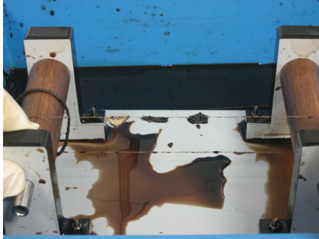
Figure 2.8. Experimental set-up for simulation of moving particles in the black ferrofluid. Note that the wooden frame is partially taken out from the tank so that it would be visible in the photo.
