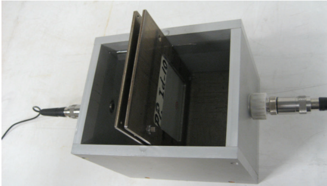
Figure 3.3. Set-up for the measurement of acoustical properties of flat polyolefin plates.
