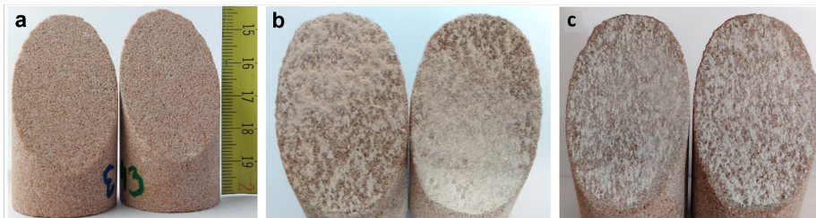
Figure 5.3: Pictures of (dried) samples before (a) and after the experiment was finished (b and c). Note that the tips of the saw-cut are ground off <3 mm, but the overall shape is still elliptical, with dimensions [45mm \pm 0.7mm / 29.6mm \pm 0.1mm] . The middle (b) shows a sample after stepwise injection and the right (c) after cyclic injection. The formed gouge is visible as the patchy whitish powder on the saw-cut fault surface. The patterns of final gouge distribution were different after each experiment, without any relationship to experimental parameters.
