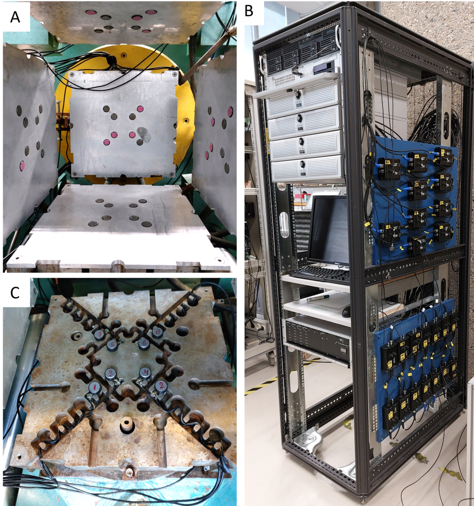
Figure A.13: Pictures showing the acoustic measurement set-up. A showing the plates with the transducers. B showing the Richter acoustic emission system, with the master computer on the top and directly below that 4 multichannel systems, below the screen the pulser amplifying system for amplification and active surveys and on the side mounted to the blue sheets, pre-amplifiers. C the bottom side, without the top-plate, showing the space for cables and transducers.
